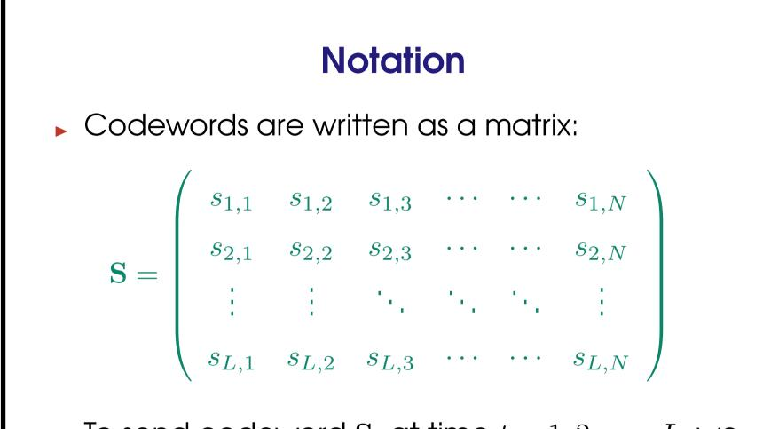
► To send codeword S, at time  $t = 1, 2, \cdots, L$ , we send  $s_{t,1}, s_{t,2}, \cdots s_{t,N}$  simultaneously from transmit antennas  $1, 2, \cdots, N$ , respectively.
