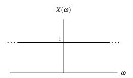
Figure 5.7: Frequency spectrum of the unit-impulse function.
