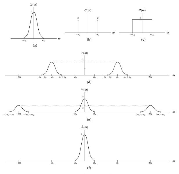
Figure 5.33: Signal spectra for DSB/SC amplitude modulation.
