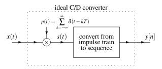
Figure 5.24: Model of ideal C/D converter.
