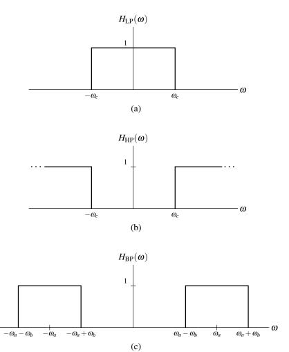
Figure 5.18: Frequency responses of systems from example.
