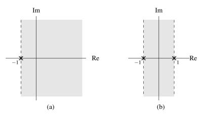
Figure 6.11: Pole diagrams for causality example.
