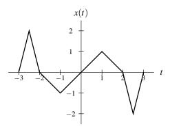
Figure 2.8: Example of an odd signal.
