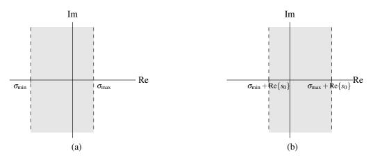
Figure 6.8: Regions of convergence for Laplace-domain shifting. (a) Before shift. (b) After shift.
