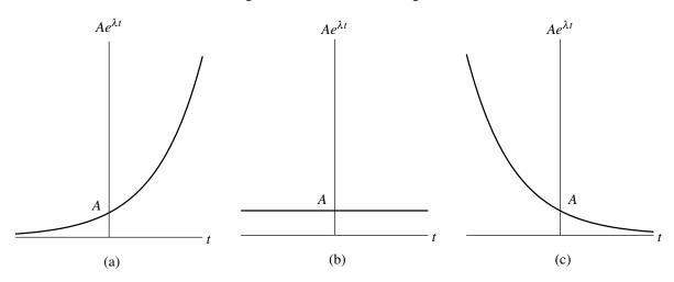
Figure 2.12: Real exponential signal for (a)  $\lambda > 0$ , (b)  $\lambda = 0$ , and (c)  $\lambda < 0$ .
