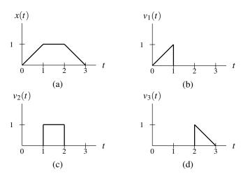
Figure 2.24: Representing piecewise linear function using unit-step functions.
