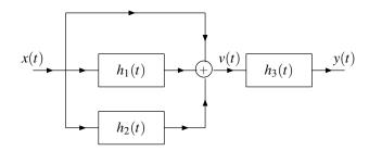
Figure 3.10: System interconnection example.
