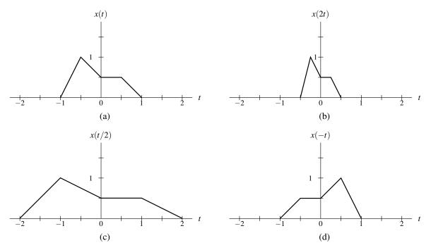
Figure 2.2: Example of time scaling.
