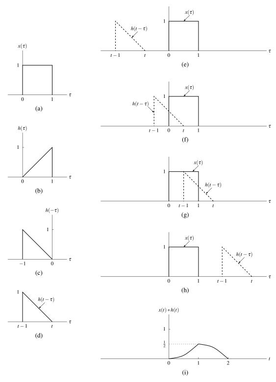
Figure 3.2: Evaluation of the convolution integral. The (a) input signal  $x(\tau)$ , (b) impulse response  $h(\tau)$ , (c) time-reversed impulse response  $h(-\tau)$ , and (d) impulse response after time-reversal and time-shifting  $h(t-\tau)$ . The functions associated with the product in the convolution integral for (e) t < 0, (f)  $0 \le t < 1$ , (g)  $1 \le t < 2$ , and (h)  $t \ge 2$ , (i) The convolution result x(t) \* h(t).
