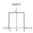
Figure 2.16: Unit rectangular pulse.
