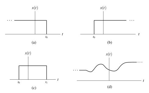
Figure 2.10: Examples of (a) left-sided, (b) right-sided, (c) finite-duration, and (d) two-sided signals.
