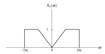
Figure 5.29: Frequency spectrum of signal  $x_1(t)$ .
