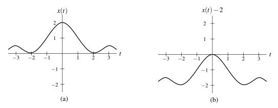
Figure 2.6: Example of amplitude shifting.
