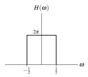
Figure 5.14: Frequency response of example system.
