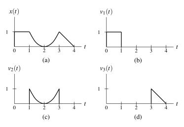
Figure 2.25: Representing piecewise polynomial function using unit-step functions.
