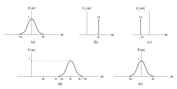
Figure 5.31: Frequency spectra for modulation with a complex sinusoid.
