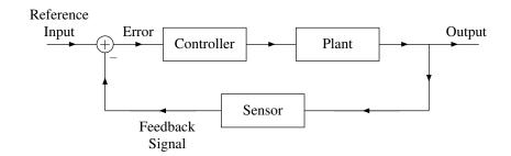
Figure 1.7: Feedback control system.
