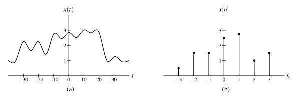
Figure 1.1: Graphical representations of (a) continuous-time and (b) discrete-time signals.
