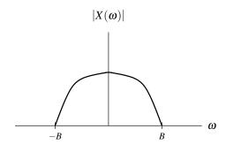
Figure 5.11: Bandwidth of a signal.
