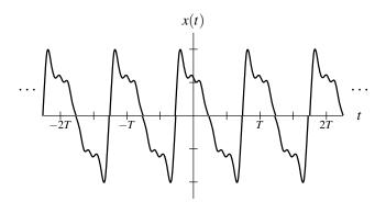
Figure 2.9: Example of a periodic signal.
