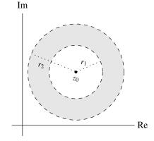
Figure A.8: Open annulus about  $z_0$  with inner radius  $r_1$  and outer radius  $r_2$ .
