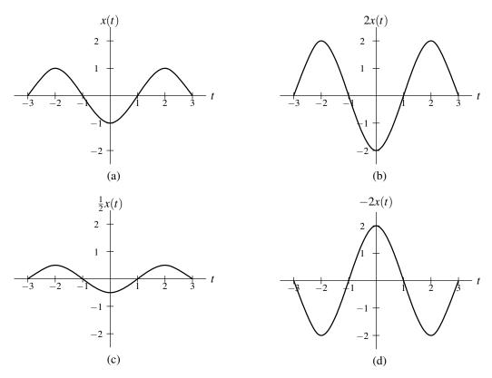
Figure 2.5: Example of amplitude scaling.
