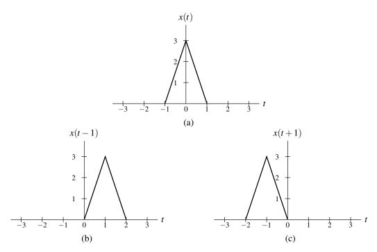
Figure 2.3: Example of time shifting.
