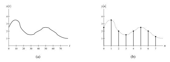
Figure 5.22: Periodic sampling of signal.
