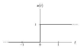
Figure 2.15: Unit-step function.
