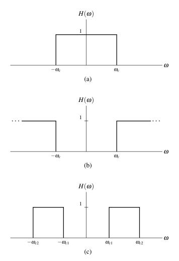
Figure 5.17: Frequency responses of (a) ideal lowpass, (b) ideal highpass, and (c) ideal bandpass filters.
