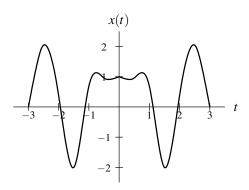
Figure 2.7: Example of an even signal.
