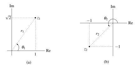
Figure A.4: Examples of converting complex numbers from Cartesian to polar forms.
