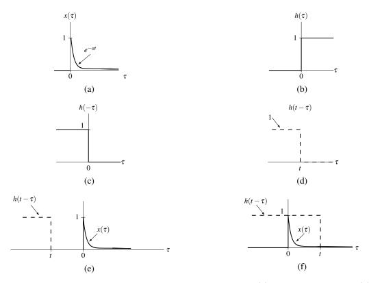
Figure 3.4: Evaluation of the convolution integral. The (a) input signal  $x(\tau)$ , (b) impulse response  $h(\tau)$ , (c) time-reversed impulse response  $h(-\tau)$ , and (d) impulse response after time-reversal and time-shifting  $h(t-\tau)$ . The functions associated with the product in the convolution integral for (e) t < 0 and (f) t > 0.
