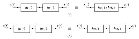
Figure 3.8: Series interconnection of continuous-time LTI systems.
